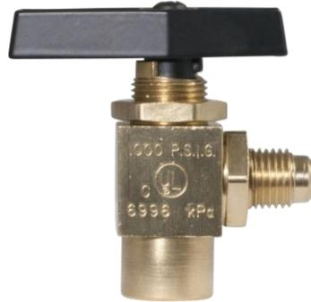
**Kantleak™** Instrumentation Ball Valves are designed with double O-ring seal providing over 20,000 cycles without leakage and an exclusive stem seal that never needs tightening. Valves can be panel mounted for instrumentation applications.
