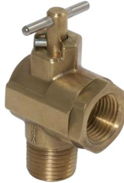
Kantleak™ Ball Valves are designed with double O-ring protection providing over 20,000 cycles without leakage and an exclusive stem seal that never needs tightening.
