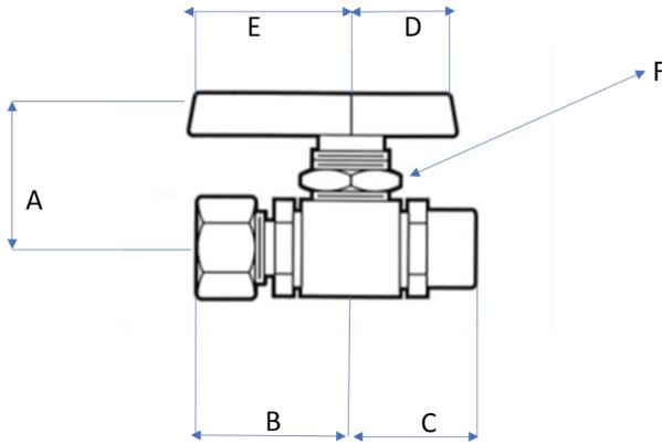
Kantleak™ Instrumentation Ball Valves are designed with double O-ring stem seals to provide over 20,000 leak free cycles. These valves also feature an exclusive stem seal design that never needs tightening and can be panel mounted for instrumentation applications.
